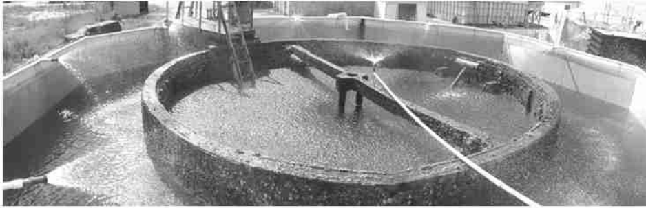
The 20-foot diameter turret -- the first turret on any warship -- sits upside-down in a constant bath of water and preserving fluids to leach out damaging salts from the iron.
